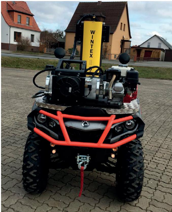
The **WINTEX 3000** is an efficient and strong automatic soil sampler. It is user-friendly, easy to use and requires only minimum maintenance. All functions are easily carried out from the driver's seat.
