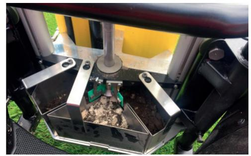
Soil from different layers is automatically filled into three soil boxes. Dividing the samples is conducted with close accuracy.
