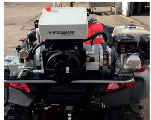
The custom-made oil tank is made of aluminum. It has a ribbed surface which means that its area is three times larger than a plain surface. Because of the aluminum and the ribbed surface the cooling capacity is 12 times higher than the cooling capacity of a traditional oil tank. This means that the tank ensures optimal cooling of the hydraulic oil.
