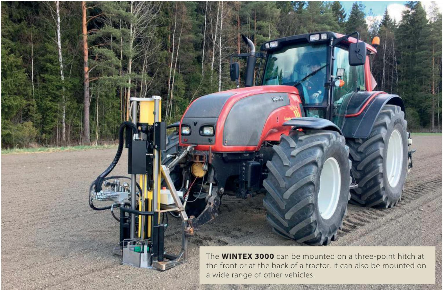
The **WINTEX 3000** can be mounted on a three-point hitch at the front or at the back of a tractor. It can also be mounted on a wide range of other vehicles.
